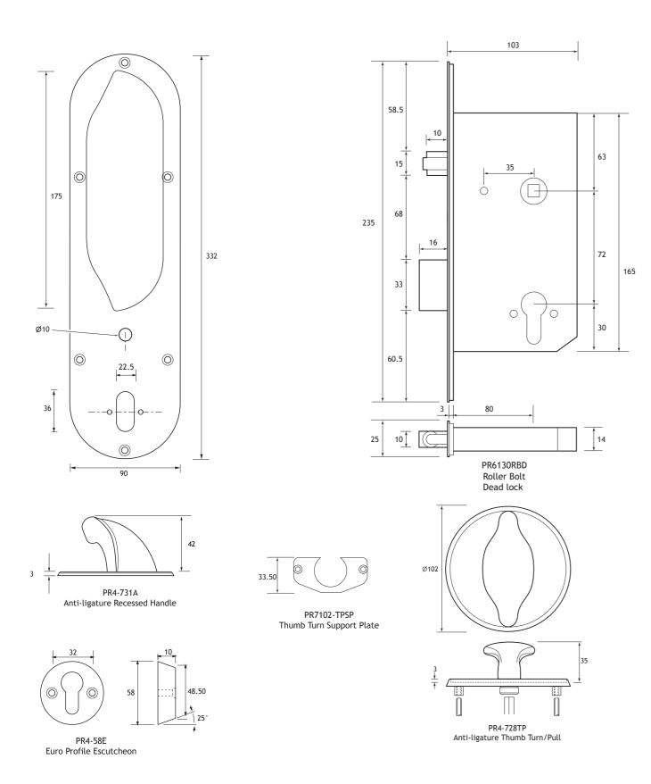
Note: The cylinder cut out is made on the external side of the door only and must not go right through the door.
