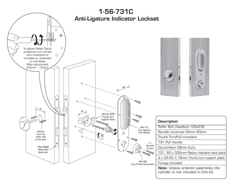
Note: If, when fitting the pull handle, the screws make direct contact with the lock-case, please use the shorter (5/8") screws included in the fixing pack.
