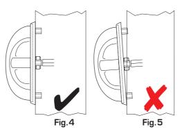
B) Cut the 2 x M5 Torx Pin machine Screws to the correct length to ensure sufficient penetration in to the Turn/Pull screw ports. If the screws are cut too long the Turn/Pull will not pull firmly back against the surface of the door resulting in a ligature risk! Secure the Turn/Pull on to the door fastening the screws through the Twin-Tech escutcheon assembly.
