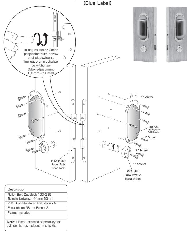
**Note:** If, when fitting the pull handle, the screws make direct contact with the lock-case, please use the shorter (5/8") screws included in the fixing pack.
