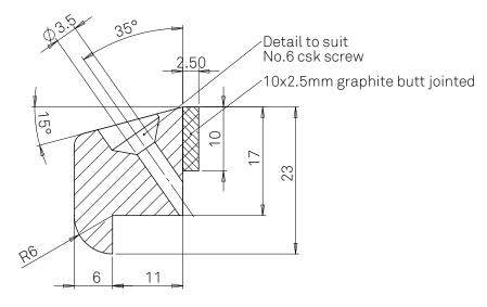
Fixing holes 50mm from corners All cassettes require 16 fixing holes
