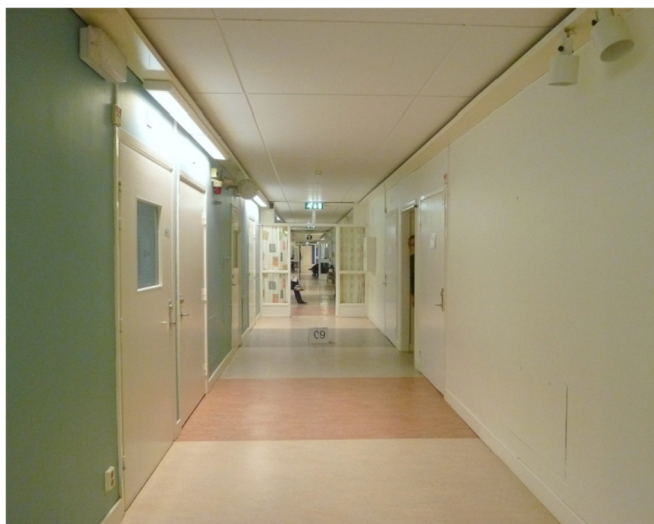
Fig. 8. Portion of a ward in Old hospital showing the corridor-dominated floor layout. The corridor-based design obstructs observation of seating and activity rooms accessed from the corridor. The photo was taken in 2010 after refurbishment for other types of patients. The hospital was subsequently demolished.
