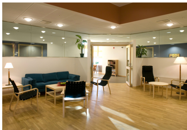
Fig. 3. Portion of a communal central area of a ward in New hospital showing groupings of movable and semi-movable seating. Half-wall partitions of break resistant glass enable staff moving in the central area to observe bedroom doors.
