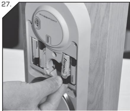
27. Insert the four AA 1.5v batteries into the battery carriers ensuring correct polarity. A red LED will illuminate.
