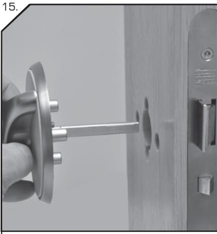
Push the Safety Spindle (5) in to Stainless Steel Turn/Pull (3A). Then, offer the Turn/Pull and spindle assembly on to the door and push the spindle through the upper follower in the lock case to loosely hold in place. Temporarily insert the external Turn/Pull spindle into the lower follower to assist with the
