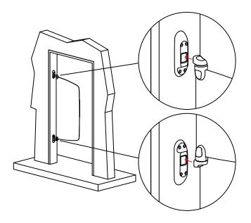
To hang the door, offer up a Door Leaf to the top and bottom Wall Mounts. It will automatically connect.
