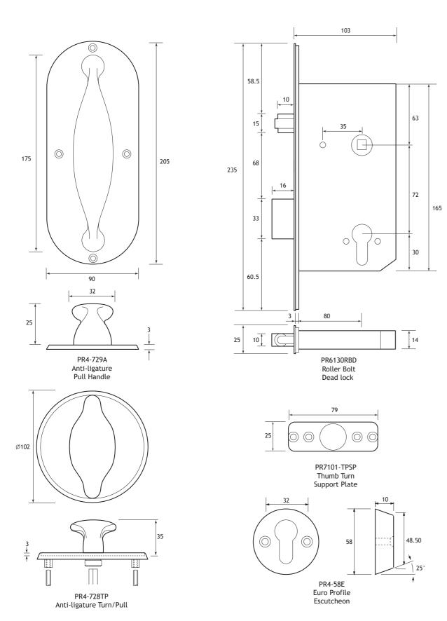
Note: The cylinder cut out is made on the external side of the door only and must not go right through the door.
