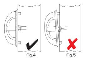
B) Cut the 2 x M5 Torx Pin machine Screws to the correct length to ensure sufficient penetration in to the Turn/Pull screw ports. If the screws are cut too long the Turn/Pull will not pull firmly back against the surface of the door resulting in a ligature risk! Secure the Turn/Pull on to the door fastening the screws through the Twin-Tech escutcheon assembly.
