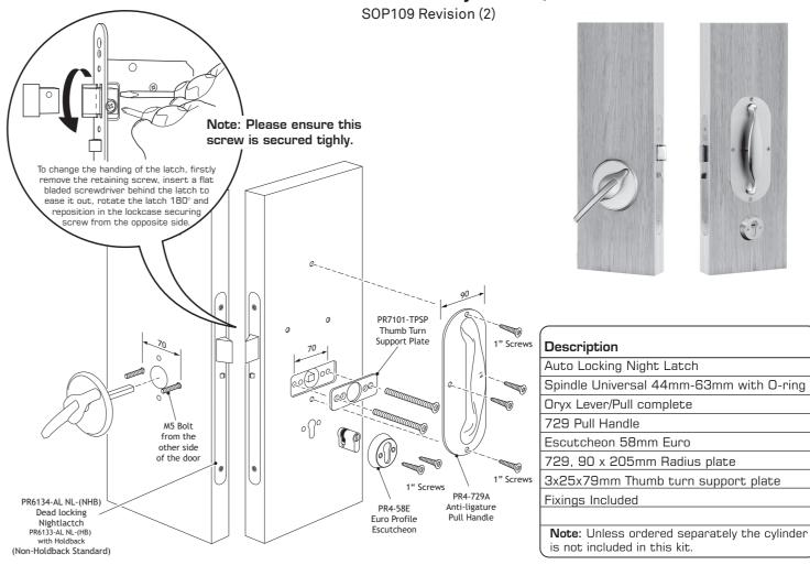
Note: If, when fitting the pull handle, the screws make direct contact with the lock-case, please use the shorter (5/8") screws included in the fixing pack.
