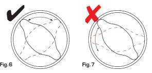
IMPORTANT: When installed correctly the Turn/Pull should not pass through the horizontal position.
