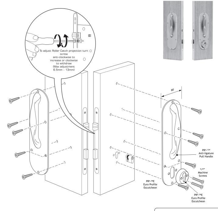
Note: If, when fitting the pull handle, the screws make direct contact with the lock-case, please use the shorter (5/8") screws included in the fixing pack.
