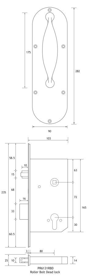
Note: The cylinder cut out is made on the external side of the door only and must not go right through the door.
