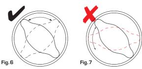
IMPORTANT: When installed correctly the Turn/Pull should not pass through the horizontal position.
