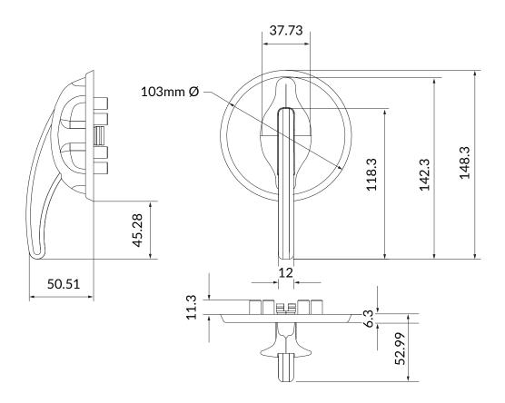
Material **Turn Rose:** Die-cast Mazak 5 handle. Electro-plated SSS finish.
