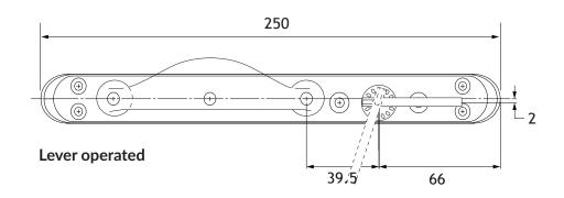
Material Handle: Die-cast Mazak 5 handle. Electro-plated SSS Finish.
