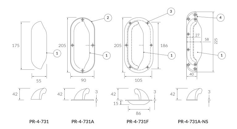
Material Handle: Die-cast Mazak 5 handle. Electro-plated SSS Finish.
