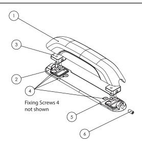
The Handle Item 1 Is Not Handed Ensure the set screw is always at the bottom of the assembly.
