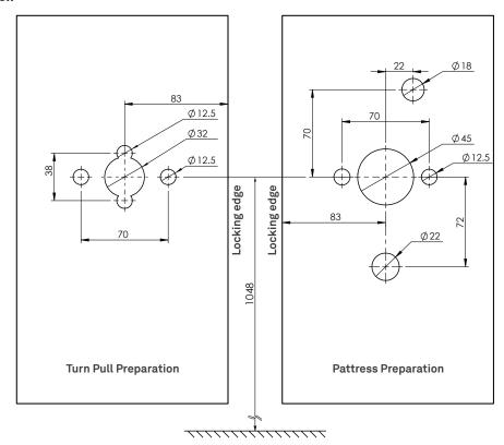
Note: 1048mm height is a recommendation. Ensure the lockset does not clash with any other door components.
