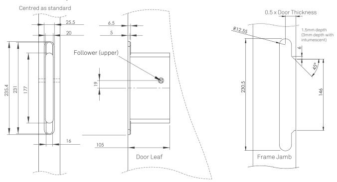
Note: 2-4mm gap between door and frame is recommended at the closing edge.
