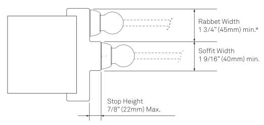
\*must leave a minimum of 3/16" (5mm) between the Wall Mount and the Soffit.
