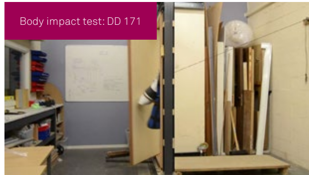
Body impact test: DD 171 Pendulum swing (EN949) to simulate a heavy body impact – up to 400J
