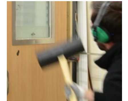
Vision panel and beading attack – to ensure robustness of the glass in the face of extreme abuse
