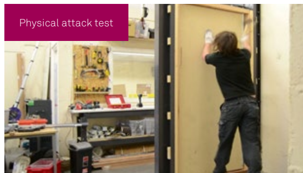
Physical attack test Department of Health UK test to simulate kicking and punching
