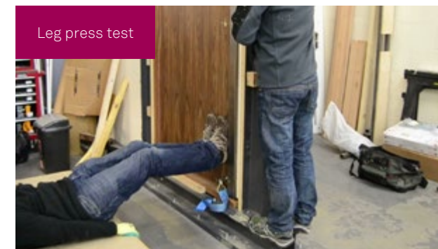
Leg press test The Leg Press test is an internal test to ensure the doorstop always releases, regardless of pressure on the stop from the inside
